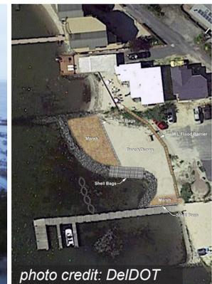
*In Pensacola, FL, "Project GreenShores," a constructed marsh with breakwaters designed to create habitat, protects a one mile segment of Bayfront Parkway from coastal erosion.*
